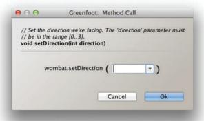
The words *int direction* tell us that this method expects one parameter of type *int*, which specifies a *direction*. A parameter is an additional bit of data we must provide for this method to run. Every parameter is defined by two words: first the parameter type (here: *int*) and then a name, which gives us a hint what this parameter is used for. If a method has a parameter, then we must provide this additional information when we invoke the method.
